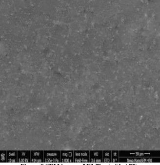
Figure 8 SEM image of F3 film (with API)
